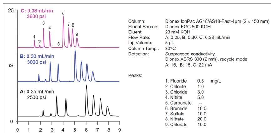
**Figure 2.** Reduction in run time achieved using higher flow rates in combination with a reduced length, 4  $\mu\text{m}$  resin particle column.
