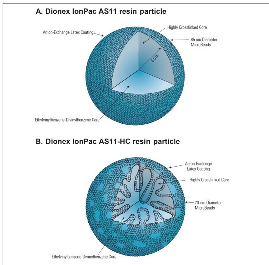
**Figure 3.** Comparison of Dionex IonPac AS11 and AS11-HC resin particle structures.
