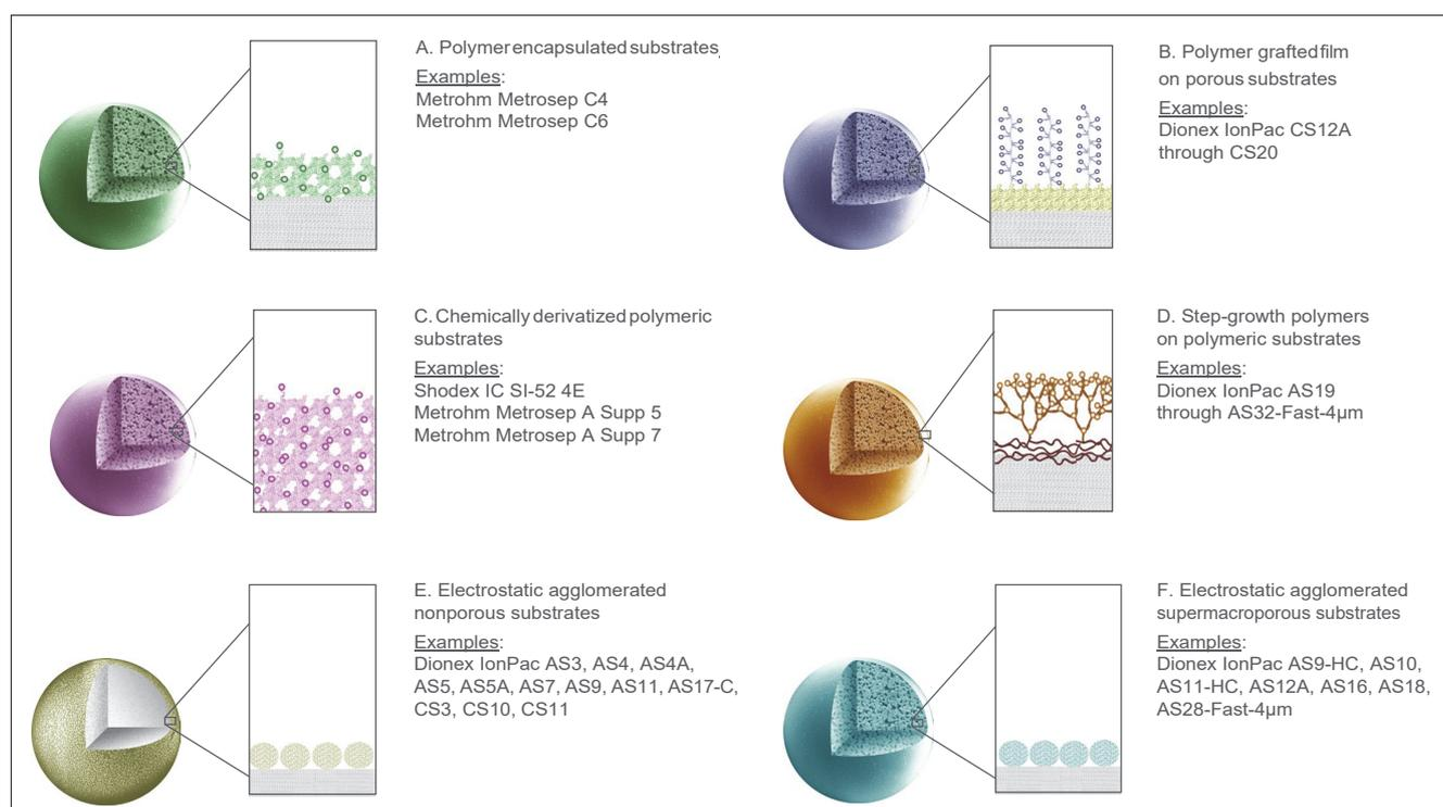
**Figure 4.** Commonly used IC column stationary-phase architectures.
