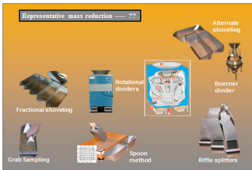
Figure 11. Overview of the principally different mass reduction methods and typical types of equipment in the authoritative benchmark study by Petersen et al. 2
