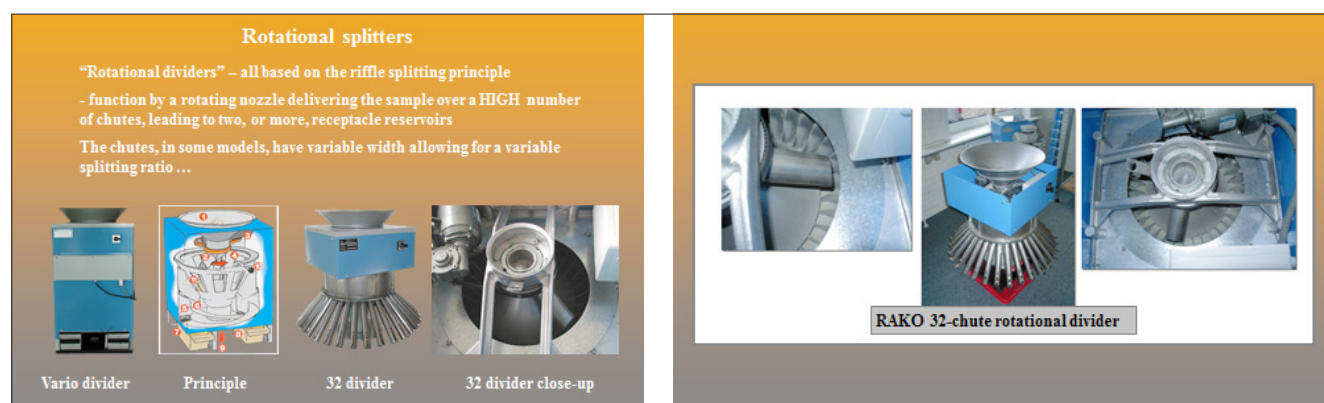
Figure 10. The rotary divider—the ultimate mass reduction equipment. Many variants of this principal solution can be automated.
