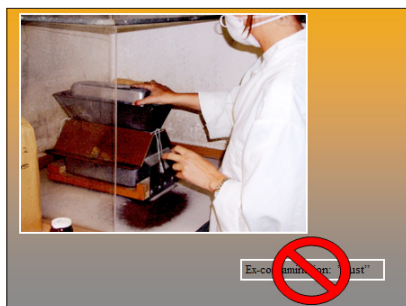
Figure 6. Albeit using only primitive and simplistic prototypes, in this analytical laboratory, the riffle splitting operations shown do everything correctly, indeed in a representative fashion: no IDE, IEE because of correct pre-loading mixing, correct loading, using a correct enclosed splitter. And should there be a residual dust fraction escaping the operations (hopefully reduced to the absolute fit-for-purpose level), a plexiglass hood has been installed (operated by a powerful exhaust fan) taking care of health risks to workers.
