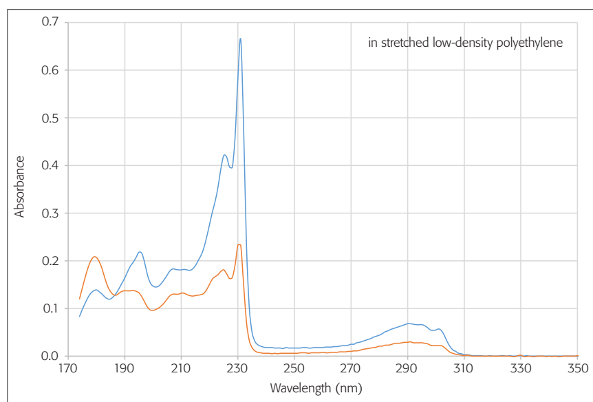
Figure 2. Linear dichroism absorbance spectrum of dibenzo- p -dioxin. 8 The absorbance curves were recorded with the electric vector of the sample beam parallel (blue line) and perpendicular (orange) to the stretching direction of the polyethylene polymer.
