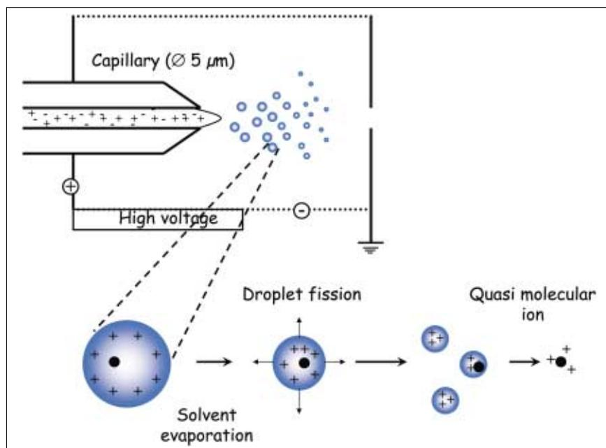
**Figure 1.** Schematic representation of the ESI process.
