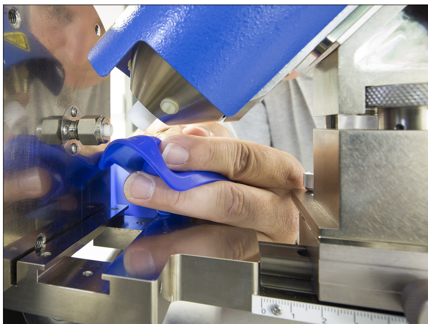
Figure 2. A silicone rubber baking mould is being subjected to positive-ion DART analysis in surface mode. The DART source (pointing down from upper right) is mounted at an angle of 45^\circ relative to the entrance of the ceramics sampling tube (left side) of the Vapur Interface. Recessing the angle mount by 20 mm (marked scale) provides enough space to manually fit the object into the ionisation zone. With the helium gas set at 300^\circ\text{C} this set-up leads to abundant PDMS ions.
