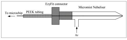
**Figure 4.** Schematic diagram of the interface [from Q. Song, G. M. Greenway and T. McCreedy, *J. Anal. Atomic Spectrom.* **19**, 883 (2004)].
