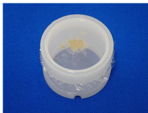
Example of very small amount of powder prepared using the film sandwich sample cup method.
