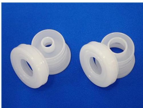
Small spot sample cups are used for pieces of small solid samples or small amount of powder.
