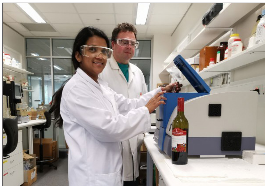
PhD student Ruchira Ranaweera loads a wine sample into a spectrofluorometer, with Associate Professor David Jeffery. Courtesy of University of Adelaide.
