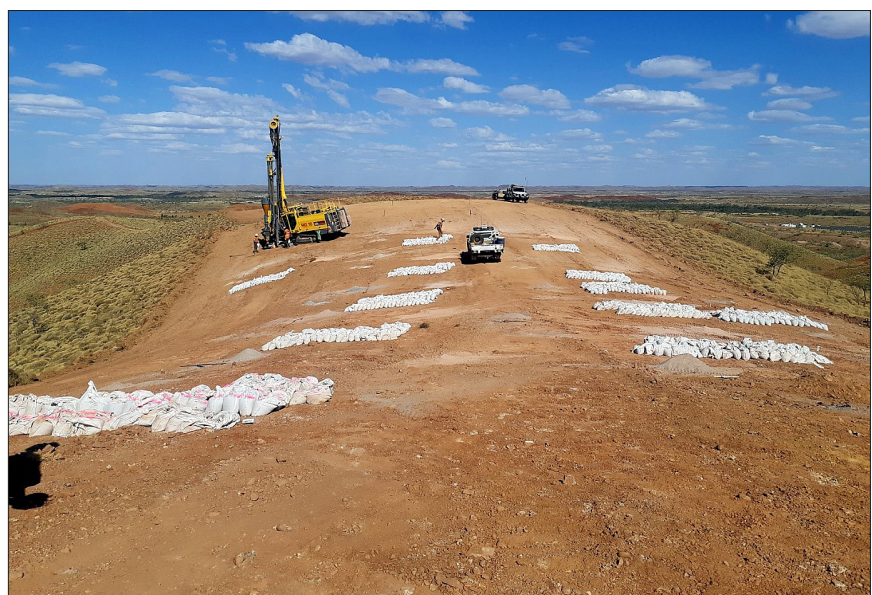
Figure 1. For optimal sampling error quantification for Gold mineral resource estimation no efforts are spared: Reverse Circulation grade control drilling at the Novo Resources Corporation Beatons Creek project in Western Australia.
