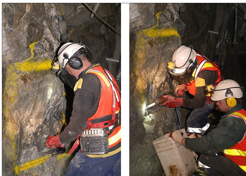
Figure 2. Underground sampling. Collection of optimal saw-cut channel sample. Left: cutting channel “delimitation” slots; right: sampling (“extraction”) of the channel material.
