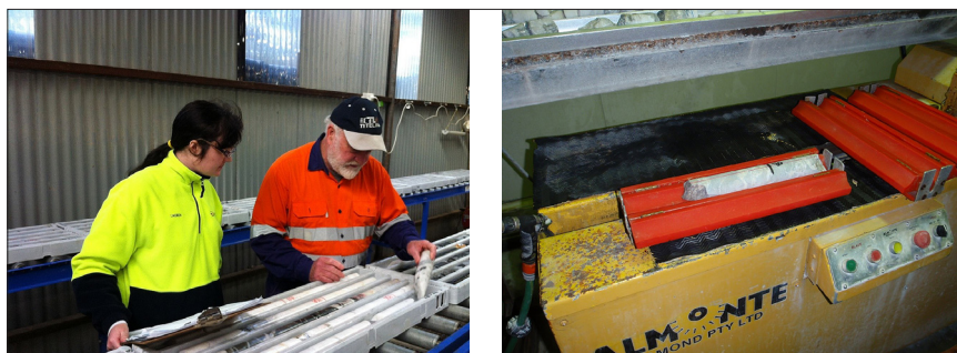
Figure 3. Left: logging and marking diamond drilling cores for sampling (at former Castlemaine Goldfields Ltd Wattle Gully project in Victoria, Australia). Right: sample preparation: diamond drilling (DD) core ready for cutting.
