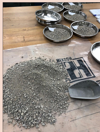
Figure 6. Soil corresponding to the PSD results shown in Figure 5. The laboratory bench pile shows a distinct constitutional and size heterogeneity manifestation. In this picture, it was undergoing sampling using MSS as defined in ASTM D6913. Samples were obtained by combining three increments grabbed from subjectively selected spots on the pile. The resulting sub-samples are seen in the metal plates in the top-right corner.
