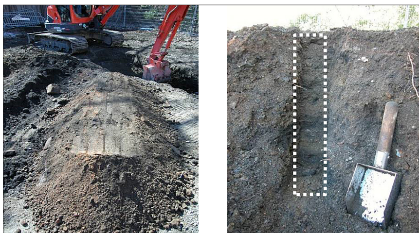
Figure 1. Left: excavated soil at a sampling station. The soil is placed in a longitudinal pile and corresponds to an identifiable layer of a given material (based on visual observation), or to a 50 cm (at most) layer if visual differentiation was not possible. Right: vertical increments are taken perpendicular to the longitudinal axis of the pile and over its total height. The primary sample mass obtained in this manner was approximately 13 kg of dry matter.
