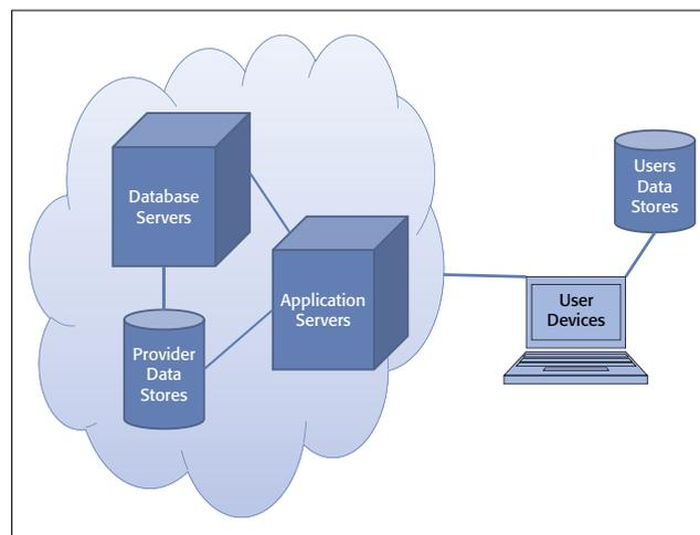
**Figure 4.** Potential hybrid model to alleviate some compliance issues around fully hosted solutions.
