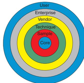
Figure 1. The Basic Shell Concept of the AnIML XML file.
